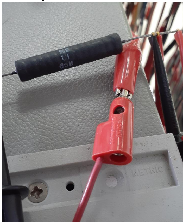
1-Ohm Shunt Resistor for measuring Current
